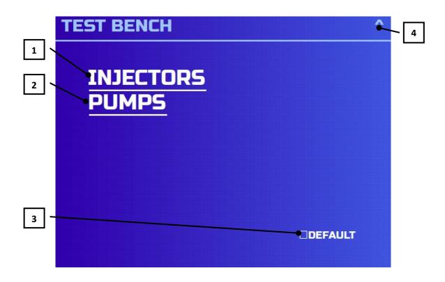
**1**INJECTORS – testing of common rail injectors on the high pressure pump bench in hand or semi-automatic mode.
