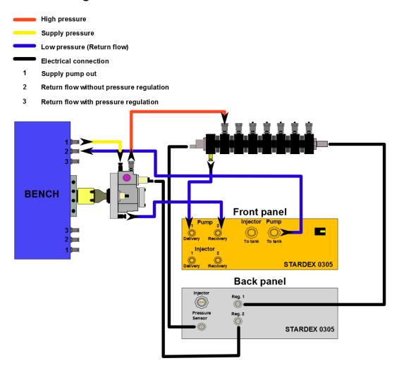
Note: while testing some Bosch CP1 pumps with the PCV (reducing valve), install the pump regulator into the fuel rail and install a special plug on its place.
